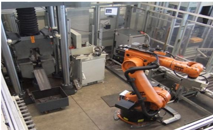
Automated tensile testing machine (1200 kN)
