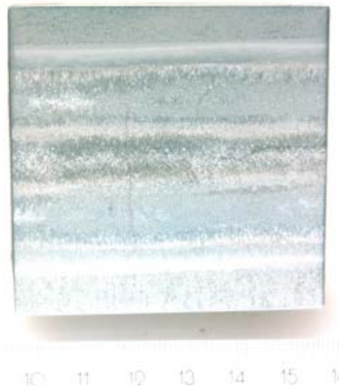
Fig. 12.2 : Positions of the cracks in the weld metal, polished surface etched in 3% nital
