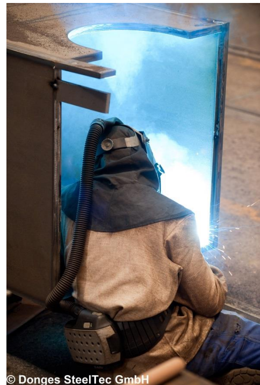
Figure 5. The reduction or even elimination of preheating makes working under constricted conditions much easier
