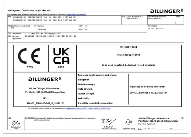
Figure 1: Example for the implementation of the CE marking and UKCA marking on certificates from Dillinger for structural steels according to the EN 10025 series of standards
