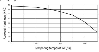
Remark: The Tempering temperature is valid for soaking time 1 h and air cooling the values in the diagram are mean values on samples, diameter 25 mm (1 in), length 50 mm (2 in), hardened at 850 °C (1560 °F) in oil
