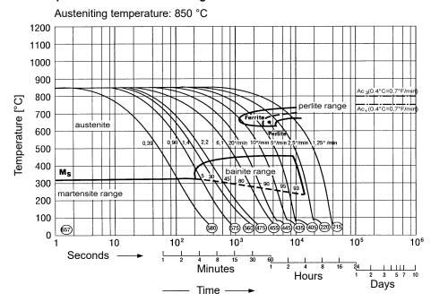
0.39 - 6.1 = cooling parameters( $t_{8/5} - time in sec./100$ )
