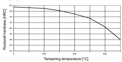
Remark: Tempering temperature is valid for soaking time 1 h and air cooling the values in the diagram are mean values on samples, diameter 25 mm (1 in), length 50 mm (2 in), hardened at 850 °C (1560 °F) in oil
